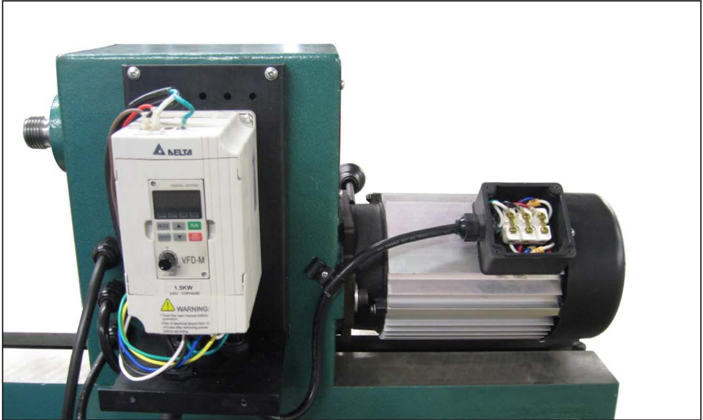
Figure 63. Inverter box and motor box locations.
